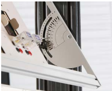
Tilttable Frame for Solar Modules with Scale
