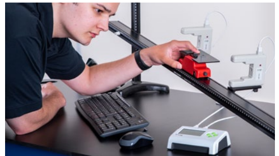
The datalogger included is fully self-contained and has a VGA output for connection to a projector for class demonstrations.
